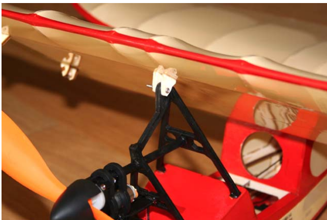
20. Fix fore wing with bolt and nut.
