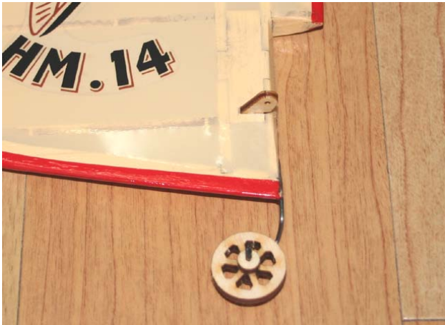
10. Insert and glue tail gear to the rudder.
