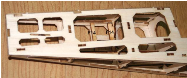
8. Glue plywood servo trays(F14) on the inner left side.
