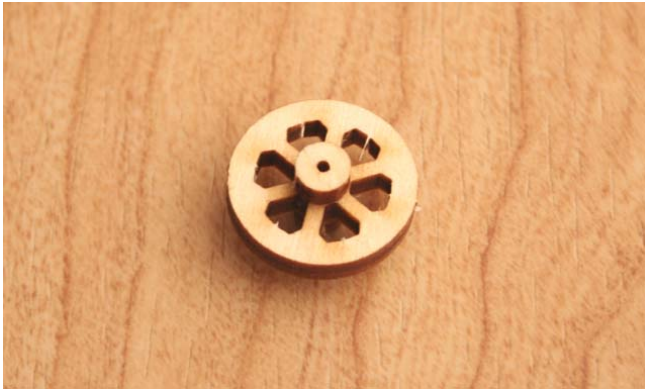
9. Assemble plywood tail wheel. Apply thin CA to the wheel for reinforcing.
