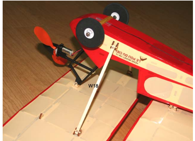
21. Attach wing strut(W18) with screws.
