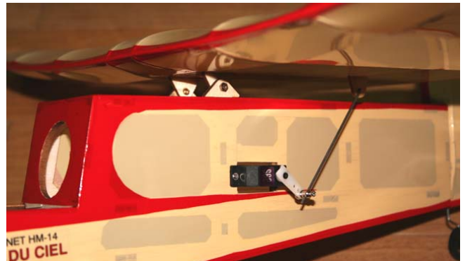
15. Fix rear wing(elevator) with bolts and nuts, and then, install elevator servo.
