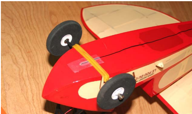
19. Fix wheels with wheel collars. Connect ESC and receiver.
