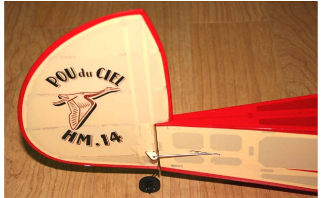
14. Connect pushrod to the rudder horn, and then, attach rudder to the fuselage by gluing hinges with small amount of thin CA.
