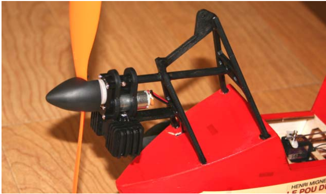
17. Install motor and gearbox, drill and fix screw to the dowel.
