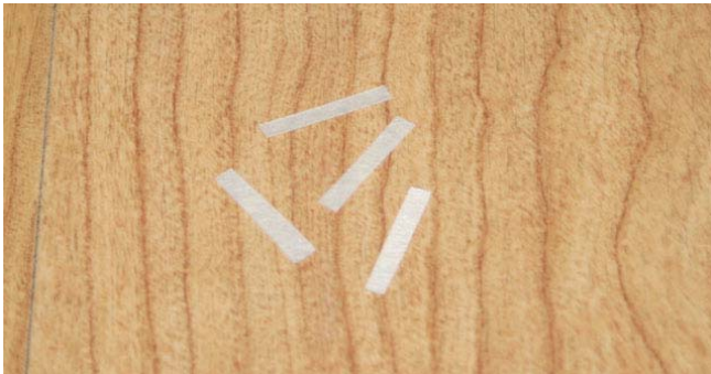
11. Cut CA hinges as shown above.
