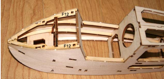
6. Insert and glue fore deck longerons(F12).
