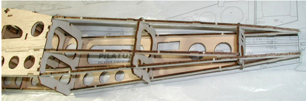
12. Temporary assemble rear longerons(F27-F28).
