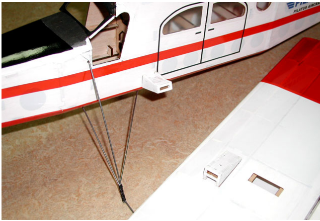
9. Insert and glue strut mounts.
