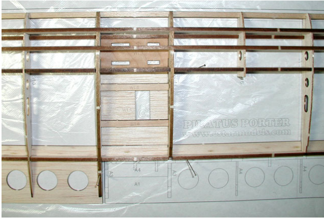
5. Assemble strut mount(W13) and servo trays(W14, W15). Pin on the plan and glue all the parts with thin CA.
