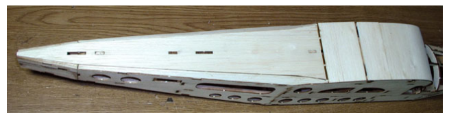
19. After sanding glue rear fuselage top cover(F45).
