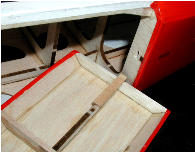
2. Glue the plywood dowel of hatch(H5).
