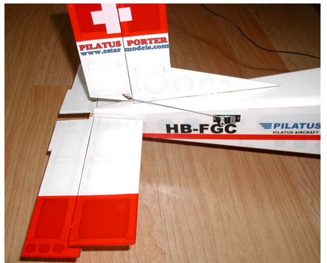
14. Install rudder servo and insert pushrods.
