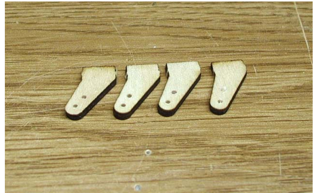
5. Prepare control horns. Drill 1.2mm holes. Apply thin CA for reinforcing.
