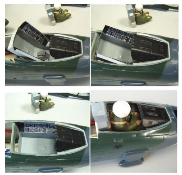
31) Try and/or modify cockpit insertion and its fixation by a magnet.
