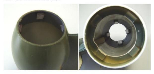
9) Install motors into blowers, connect regulator wires, prepare extension cables and V cable for regulators connection. Set up all RC equipment with motors "on the table" and test correct functions of motors, regulators and servos before installation into the model.
