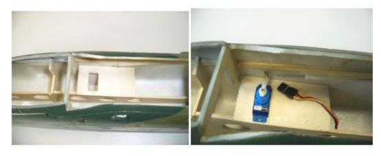
48) Connect the link with micro lever 61 at elevator 6 and with servo in fuselage. ATTENTION! Elevator shall not have clearance due to partial blowing by blowers!!
