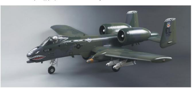
The A-10 Thunderbolt II was the first plane of American Air Force designed especially as ground attack aircraft for direct support of ground army units. It is a simple, effective and robust jet aircraft with two engines that can be used against all ground targets including tanks and other armored vehicles. The fundamental means is dreaded 30 mm rotational cannon GAU-8/A of Avenger Gatling type.
