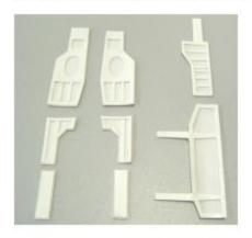
53) Stick doors of landing gear shafts to shafts. Door braces can be made from steel wire.
