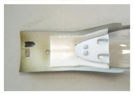
27) Set up pilot figure 23, adjust instrument panel 28, instrument panel cover 33, cockpit interior 35 and pilot seat 31. Apply instrument decals.
