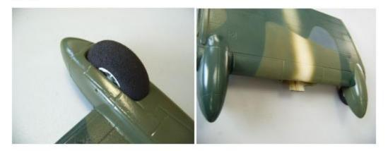
37) Stick aerodynamic panels 12 to leading edges of center-wing. Then proceed from point 42.
