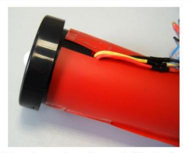
(1) Remove ring covers from nacelles, remove front fairing from blowers. You can glue spinner 22 on ducted fan.
