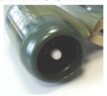
17) Cover for ventilation of regulators 30 between nacelles can be equipped with locks from PSH strips for access to regulators or can be glued firm.
