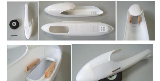
36) Insert wheels **40** into shafts and insert wheel axles **52** without using glue. Glue nacelles to center-wing section **3**, do not interchange left and right nacelle. Cut off polystyrene in center-wing section **3** in position of wheel axle plates.
