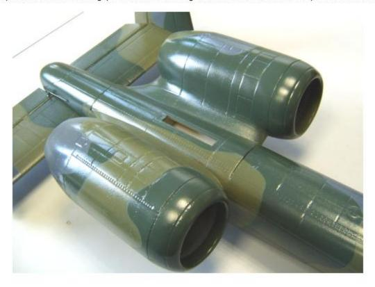
56) Stick center-wing section into fuselage cutout, glue plastic fairings 19 fuselage -- center-wing section.
