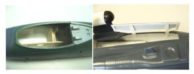
40) Stick assembled locks of landing gear legs to center-wing section, at the same time stick rear wedges 54 between center-wing coverings. Observe correct positions of locks.
