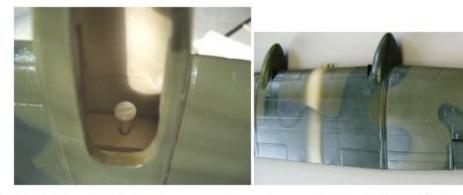
47) Glue bulkhead **42** into fuselage and install servo for elevator. Run steel wire (link) through bowdens. At the same time modify both ends of bowden in position of connection of both parts **1** and **2** of fuselage.
