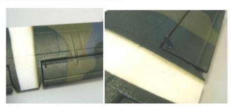
3) Glue right vertical stabilizer 7P to right side of horizontal stabilizer 6. Insert horizontal stabilizer 6 into cut out from right side, check free movement of elevators, glue it from inside of fuselage and glue left vertical stabilizer 7L.
