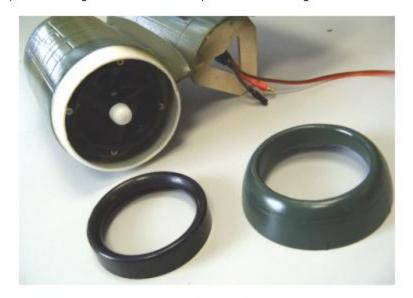
12) Insert jets with blowers into nacelles and at the same time run wires with regulators through and screw blowers to glued plates 58 on bulkheads. Jet ends shall be directed upwards.
