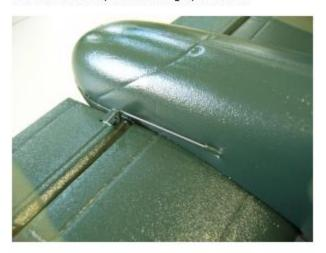
49) Stick ground balsa plates 65 to both halves of landing gear legs 16 and prepare grooves for steel wire 50 in them. Make hole of 2 mm dia in marked positions of both moldings for shaft 50 insertion. Glue steel landing gear legs 50 in grooves, glue both parts together.
