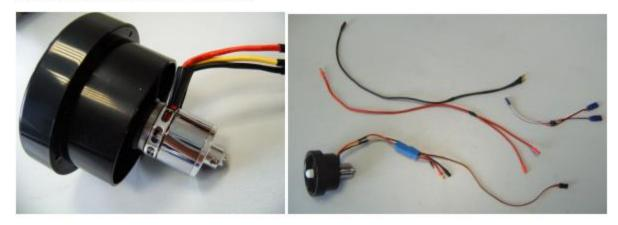
10) Try insertion of jets on blowers 18 and make cut outs for leading motor cables from jets.
