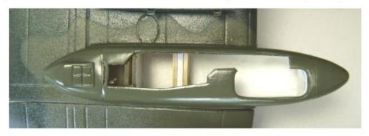
42) Stick servos in frames 43, connect extension cables and stick them into shafts in wings - run cables out of wings. Glue balsa pads between servo frames and shaft bottoms if necessary.
