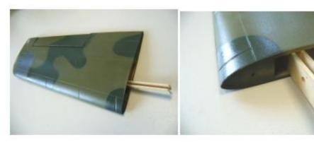
46) Connect wings with center-wing section, screw them with screws 45 by landing gear shafts, do not forget to run wing servo cables into center-wing section. This operation can be made during final model assembly. You can fasten wings with center-wing section firmly if you do not need removable wings.
