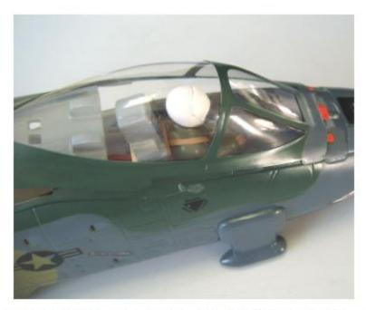
32) Try insertion of batteries, determine their position after assembly of complete model so that it would correspond to the center of gravity. There are two polystyrene bulkheads inserted in fuselage that would be glued when battery pack position is determined.
