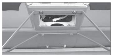
$\Box$  3. Attach the landing gear to the bottom of the fuse with four 2mm x 7mm [5/64" x 9/32"] self-tapping washer head screws. Remove the screws and harden the holes with thin CA. Then, reinstall the screws.
