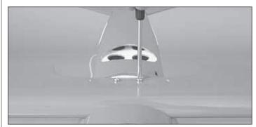
□ 2. Place the middle wing on the wing saddle as shown and secure it with two  $3mm \times 24mm [1/8" \times 15/16"]$  machine screws and 3mm [1/8"] washers. The flat side of the wing is the bottom.
