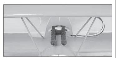
□ 1. Remove a 13mm x 13mm  $[1/2" \times 1/2"]$  square of covering from the top of the fuse in front of the cockpit and use CA to attach the machine gun mount. Glue the machine guns in place as shown.
