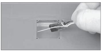
**TIP:** After tying the string to the right aileron servo plug, use tape to keep the string and plug headed in the same direction. This accomplishes two things; it keeps the plug from doubling back over itself and keeps the string securely fastened to the plug.
