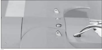
□ 3. Grab the two strut mounts that you marked "B" and insert them into the pockets on top of the middle wing as shown. **DO NOT** glue them into place at this time.
