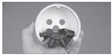
$\Box$  2. Use Medium CA to glue the dummy engine in place on the cowl as shown.
