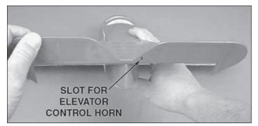
□ 9. Temporarily attach the elevator to the stab with four CA hinges. **IMPORTANT:** There is a left and right side to the elevator. The bottom, right side of the elevator has a small slot for the elevator control horn. **Be sure the elevator half with the slot is on the bottom, right side of the fuse.** Use T-pins to hold the CA hinges centered in the elevator as you did when installing the ailerons on the Top wing. Apply 3 drops of thin CA on the top and bottom of each hinge.
