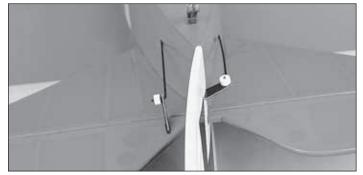
□ 3. Insert the 90° bends of the 460mm [18"] pushrods into the outer hole of the control horns and secure them with the plastic retainers as shown. Place a drop of CA on the outer surface of the plastic retainers.
