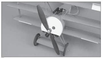
$\Box$  3. Install a 10" x 4.5" propeller. Install the prop washer and prop nut and tighten the nut securely.
