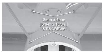
□ 4. Locate the two cabanes and install them as shown using four  $2mm \times 6mm [5/64" \times 15/64"]$  self-tapping screws as shown. Remove the screws and apply a couple of drops of thin CA into each hole to harden the threads. Re-install the cabanes.
