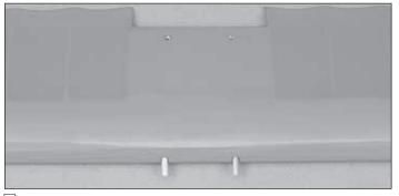
□ 1. Locate two of the 3mm x 24mm  $[1/8" \times 15/16"]$  dowel rods and insert them into the bottom wing as shown, so that only about 9mm [11/32"] sticks out. Secure them with medium CA.
