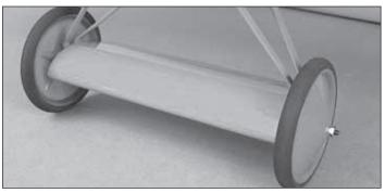
□ 4. On each end of the axle, place a 3mm [1/8"] washer and 3mm [1/8"] nut with threadlocker, followed by another 3mm [1/8"] washer and the wheel. Secure the wheel in place with a 3mm [1/8"] washer and 3mm [1/8"] nut. Apply a drop of threadlocker to the nut.
