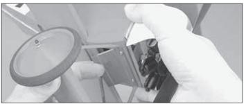
$\Box$  2. Put the battery cover in place. Note that the lip slides into the fuse and the aft end is held on with two magnets.
