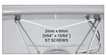
□ 5. Put the top wing in place atop the cabanes and secure it with four  $2mm \times 6mm$  [5/64" x 15/64"] self-tapping screws. Remove the screws and apply a couple of drops of thin CA into each hole to harden the threads. Re-install the top wing.
