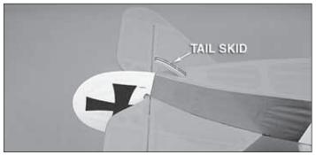
$\Box$  11. Test fit the tail skid at the rear of the fuse. When satisfied with the fit, attach the tail skid to the bottom of the fuse using medium CA.
