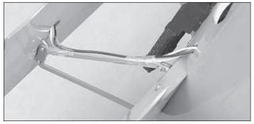
□ 3. Use clear tape to secure the aileron wire to the cabanes as shown and hide the wire with the included segment of red covering material.
