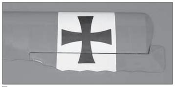
□ 2. Remove any pins you may have inserted into the hinges. Install the aileron so there is a very small gap between the LE of the aileron and the wing. The gap should be small – just enough to see light through or to slip a piece of paper through.
