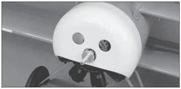
$\Box$  2. Slide the prop shaft and collet onto the motor shaft. The collet has a tapered hole through it.
