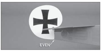
□ 10. Install the 10mm x 21mm [3/8" x 13/16"] CA hinge in the rudder and test fit it into the rear of the fuse. Adjust the rudder so that the bottom is even with the bottom of the fuse. Use a small modeling square to make sure that it is perpendicular to the stab. Apply 3 drops of thin CA on each side of the hinge.
