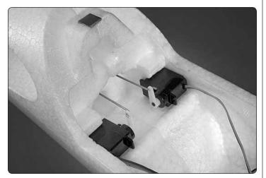
☐ 6. Install the pushorods through the guide tubes in the fuselage. Then, connect the pushrods to the outer holes in the servo arms. Glue the servos into position.
