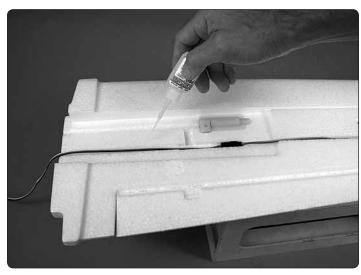
☐ 7. Glue the bottom wing cover into position—thick or medium CA is okay here, but *use care* not to allow any glue to leak into the channel or into the clamp for the joiner tube. If necessary, use tape or weights to hold the cover down until the glue hardens.
