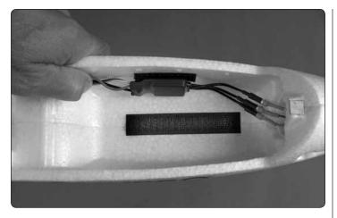
4. Apply a strip of the rougher, "hook-side" of the hook-and-loop material to the bottom of the radio compartment for the battery. Apply thin or medium CA all the way around the edges of the strip to make certain it is adhered permanently.
