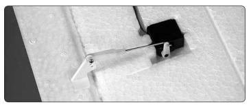
2. Without using any glue, temporarily fit the servos into the pockets in the wing. Hook up the ailerons with the hardware shown.
