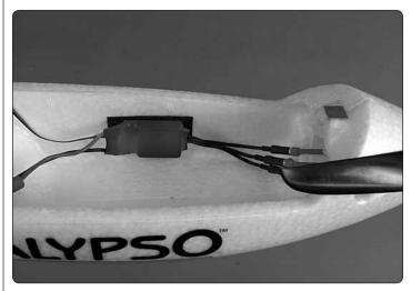
□ 3. Connect the ESC to the motor and mount the ESC to the inside of the fuselage with strips of the included adhesive-back hook-and-loop material. **Note:** If, while running up the motor later, the propeller turns backward, simply switch any *two* of the three motor wires with each other to make the motor turn the other direction.
