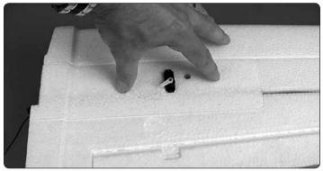
☐ 5. Without using any glue, test-fit the bottom wing cover to the wing. Make sure the cover lays all the way down flat into the cavity and make any adjustments necessary.
