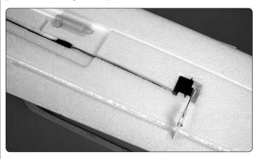
□ 3. Connect a 18" – 24" [460mm – 610mm] servo extension to the aileron servo wires and secure the connection with tape,
