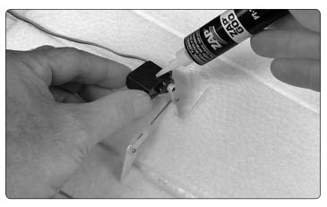
☐ 6. Glue the aileron servos (and flap servos if installed) into position—thick or medium CA is suitable, but if ever necessary, the servos will be easier to extract later if something more flexible such as Zap Goo or similar is used.
