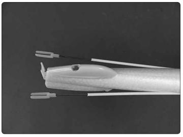
7. Thread the clevises onto the pushrods until the end of each pushrod protrudes through the clevis just enough to become visible.
