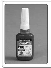
Non-permanent threadlocker should be used on all screws that thread into metal such as the motor mount screws, the set screws in the propeller hub and the screws that secure the spinner—a large amount of threadlocker is not required—just enough to "wet" the first few threads.
