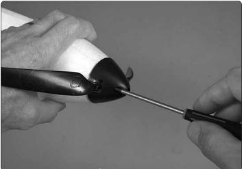
2. Fasten the propeller hub onto the motor shaft using a 1.5mm hex wrench to tighten the set screws. Then, mount the spinner with the 3 x 12mm screws.
