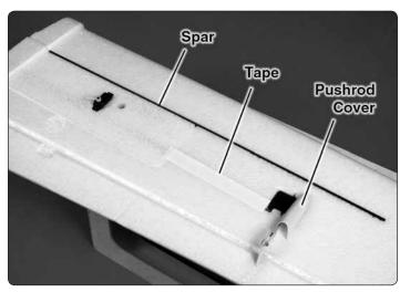
□ 8. Glue the spars and optional aileron pushrod covers into position. Also apply a strip of white or clear tape over the channel for the aileron servo wire.
