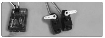
☐ 1. Temporarily connect the aileron servos and ESC to your receiver and turn on your transmitter. Making sure the trims on your transmitter are centered, connect the battery to the ESC. If necessary, remove and re-mount the servo arms so they will be perpendicular as shown. Be certain to replace the servo arm screws.
