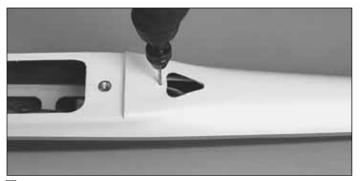
□ 2. Drill a small hole as shown for the antenna to exit the fuse. Do not route the antenna inside the carbon fiber fuselage!
