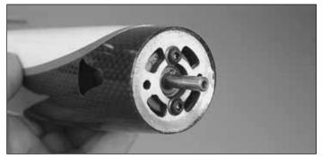
□ 2. Guide the motor into the nose of the airplane from the inside of the fuselage. Secure the motor to the firewall using screws provided by the motor manufacturer and thread-locking compound.
