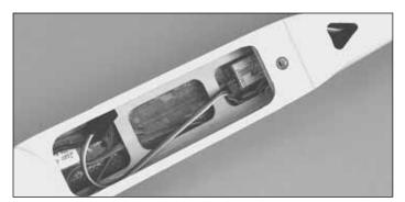
□ 1. Connect the elevator, ESC, and aileron Y-harness to the receiver. Mount the receiver in the rear of the radio compartment with double-sided tape.
