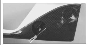
☐ 7. Center the servo and attach the clevis to the servo arm. Shift the servo to get the elevator neutral and the top of the servo parallel with the pushrod.
