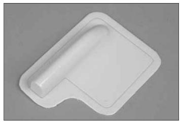
□ □ 7. Carefully trim the servo cover along the cutlines. Lightly sand the area of the heat shrink servo wrap that will be glued to the wing. Align the servo so that the pushrod clears the cover. The servo travel should not bind against the servo cover. When you have everything lined up, glue the servo in place using epoxy.
