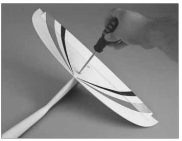
□ 1. Inspect the hinges and the hinging motion of the elevator now and before each flight. Cut the 10-24 x 2" [52mm] nylon bolts to 3/4" [19mm] long. Attach the stab to the fuse using the two nylon bolts. Be careful not to overtighten.
