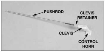
□ □ 4. Thread a nylon clevis twenty turns onto the threaded end of a 2mm x 150mm threaded pushrod. Slide a clevis retainer over the clevis. Attach the clevis to the outer hole of a small nylon control horns.
