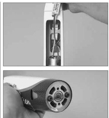
$\Box$  2. Guide the motor into the nose of the airframe from the inside of the fuselage. Mount the motor to the firewall using the screws that came with the motor and Threadlocker.
