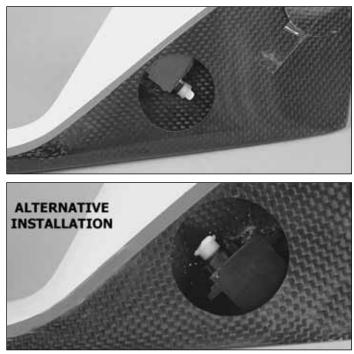
□ 5. Temporarily position the elevator servo as shown. Use fine-grit sandpaper to sand the area on the fuselage and heat shrink wrap where the servo will be glued. **Note:** Alternatively the servo can also be installed right-side up.
