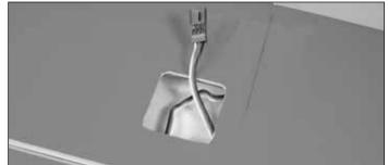
$\Box$  2. Connect the servo lead to the 24" [610mm] servo extension. Secure the connection with a 1-1/2" [38mm] piece of
