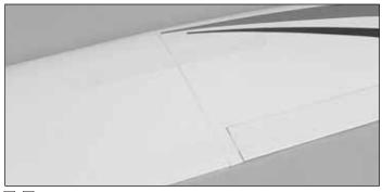
□ 3. Cut away the covering from the servo bay. Using 30minute epoxy, coat the wing joiner, wing center-section rib, and wing outer panel. Attach the wing outer panel. Route the servo extension from the center-section into the servo bay. Clean up any excess epoxy with denatured alcohol and a paper towel. Align the trailing edge of the center-section and the outer panel. Hold the two in place using masking tape while the epoxy hardens.
