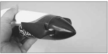
□ 3. Check for proper motor rotation. Attach the prop adapter, prop, and spinner to the motor shaft as determined by your manufacturer.
