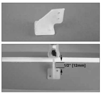
□ 2. Cut the remaining small control horn as shown. The horn is installed centered on the opening in the top of the fin and the base of the horn is 1/2" [12mm] back from the hinge line. Install the control horn using two 2-56 x 5/8" [16mm] bolts and the nylon backplate. Remove the stab from the fuselage.
