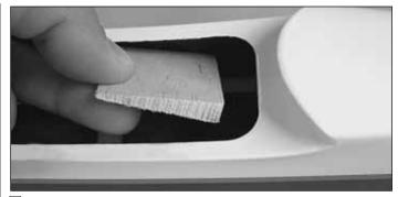
□ 4. If the battery does not slide forward far enough to fit inside the fuselage, tack glue the hardwood wedge on the battery tray against the forward former. This wedge will lift the front of the battery and it will help it slide through the forward former easily.
