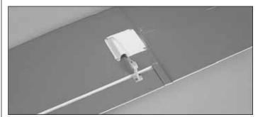
$\Box$  8. Mark the location of the servo cover screws on the wing. Drill a 1/16" [1.6mm] hole at that location. Harden the
