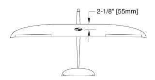
□ 2. With the wing attached to the fuselage and all parts of the model installed (ready to fly), place the model on a Great Planes CG Machine<sup>™</sup>, or lift it at the balance point you marked.
