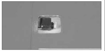
□ □ 3. Temporarily attach the servo to the receiver. Turn on the radio and center the servo. Test fit the servo in the servo bay. Adjust the servo arm until one of the arms is at a 90° angle to the bottom of the wing. Cut off the remaining servo arms and tack glue the servo in place with a drop of medium CA.
