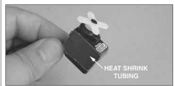
□ □ 1. Using a piece of Trinity Single Cell heat shrink tubing, fit the tubing over the servo and heat shrink it. This will allow you to easily replace the servo later since the tubing will be glued in place, not the servo.
