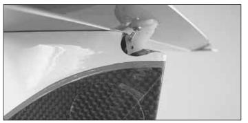
□ 9. It may be necessary to widen the opening in the top of the fin, or to remove a portion of the opening to allow the pushrod to travel.
