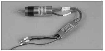
□ 1. Connect the motor to the ESC following the manufacturer's instructions.
