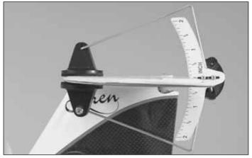
Use a Great Planes AccuThrow<sup>™</sup> (or a ruler) to accurately measure and set the control throw of each control surface as indicated in the chart that follows. If your radio does not have dual rates, we recommend setting the throws at the **middle of both rate settings**.
