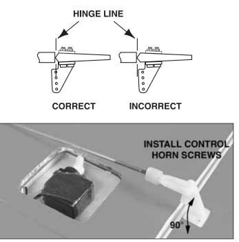
□ □ 5. Align the holes in the control horn with the hinge line, keeping the pushrod aligned with the servo arm. Mount the
