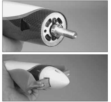
□ 3. Check for proper motor rotation. Attach the prop adapter, adapter washer, prop, and spinner to the motor shaft as determined by the motor manufacturer.
