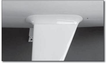
□ 2. The main landing gear leg fairings are only slightly different. It is difficult to see the difference by just looking at them. We recommend test fitting both of the landing gear fairings over the main landing gear and checking the fit. If they are properly oriented, they should fit against the fuselage closely. If they do not, try switching them or rotating them front to back.
