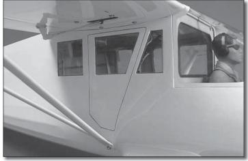
4. We have also included a template for the passenger door. Turn to the back of this manual and cut this out. Hold it up to the right hand side of the model and trace the outline of the door onto the fuselage using a panel line pen.
