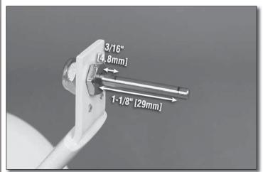
□ 4. Install an axle onto a landing gear leg using a 5/16-24 lock nut. Using a felt tipped pen, mark the bottom side of each axle as shown. Make one mark 3/16" [4.8mm] from the base of the axle and the other mark 1-1/8" [29mm] from the base of the axle.
