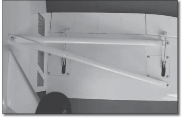
□ 3. Turn the model over and install the wing struts onto the wing and the fuselage using three 2-56 x 1/2" [12.7mm] machine screws, three #2 lock washers, and three #2 flat washers. Add a bit of thread locking compound to the screw threads for added security. Lay the front strut over the rear strut at the fuselage attachment point. Then, install the screw.
