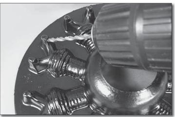
□ 2. Pushrod tubes are provided for you if you choose to detail the dummy engine. Drill a hole in the bottom of the rocker cover and a corresponding hole in the crank case using a 3/32" [2.4mm] drill. To start the hole, use your hobby knife and poke a small "starter hole" to keep your drill centered.
