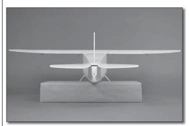
□ 4. Raise and support the tail of the model and take a few steps back. Look at the alignment between the horizontal tail and the wing. If one side of the tail sits higher than the other,
