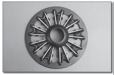
□ 4. Use a sharp hobby knife or small sanding drum to remove the plastic between the dummy engine cylinders. Leave a 20mm wide ring around the edge of the dummy engine. Use sand paper to remove the paint from the lip of the dummy engine. Clean the lip using denatured alcohol.
