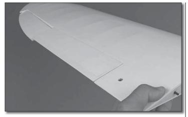
□ 3. Mix up a batch of 6-minute epoxy. Brush epoxy on the leading edge of each flap and the corresponding trailing edge of each wing. Glue each flap in the retracted position. Before the epoxy cures, wipe off the excess with a paper towel dampened with denatured alcohol.
