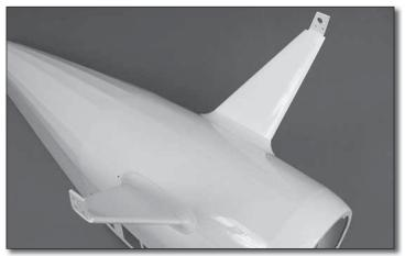
□ 3. Glue the fairings to the gear legs using R/C-56 canopy glue around the flange. Clean up any excess glue with a damp paper towel. Tape the fairings in place. Remove the tape after the glue dries.
