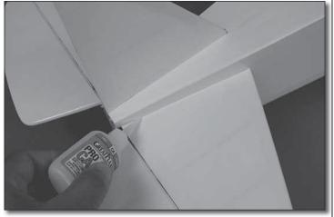
□ 6. Pull the vertical fin out of the fuselage. Using a toothpick apply 30-minute epoxy to the top of the horizontal stabilizer, through the vertical fin slot. Glue the horizontal and vertical tail to the fuselage using thin CA. Wick several generous beads of CA into the tail to fuselage joints. Remember to apply glue to both sides and the top and bottom of the horizontal stabilizer.
