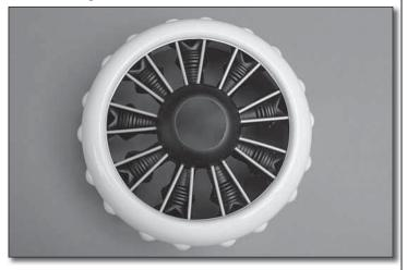
□ 6. Fit the dummy engine inside the cowl. Position it as far forward as possible, aligning the rocker arm covers with the blisters on the cowl. Apply epoxy along the seam between the dummy engine and the cowl.
