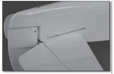
□ 2. Fit one pushrod into the elevator pushrod guide tube on the left side of the fuselage.
