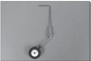
□ 1. Clean the surface of the plastic tailwheel bushing using denatured alcohol. Sand the bent portion of the tailwheel wire. Apply a drop of oil onto the tailwheel wire to prevent the wire from being glued to the bushing.
