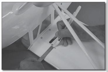
□ 1. Turn the model over and mark the C.G. location on the bottom of the wing using a felt-tip pen. The C.G., or balance point, is located at 2-1/4" [57mm] back from the leading edge of the wing at the wing root. This is where your plane should balance and fly for the first few flights. Note: It is permissible to fly the airplane with the C.G. up to 1/4" [6.4mm] forward or 1/4" [6.4mm] aft of this point. Do not fly outside of the listed C.G. range!
