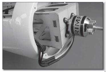
□ 9. Test the motor for proper operation. If the motor does not spin in the correct direction, unplug two of the motor wires from the ESC and swap the position of the two wires. Test the motor once again to confirm. **Warning:** Do not install the propeller until you have performed this check and have determined that the motor works properly.
