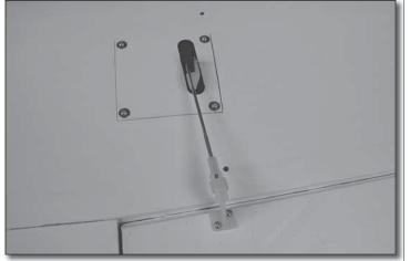
□ □ 12. Bend the pushrod 90° at the mark that you made. Fit the pushrod to the servo arm and fasten it with a FasLink pushrod retainer. Cut off the remaining pushrod so that at least 1/4" [6.4mm] of pushrod remains.
