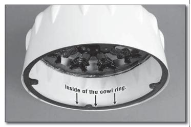
□ 11. Once the epoxy has cured, remove the cowl and plastic bag. To increase the strength of the joint between the cowl and cowl ring, apply a small fillet of epoxy on the inside of the cowl ring.
