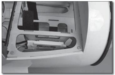
□ 7. Glue the ESC tray into the fuselage as shown. Fit the ESC. Connect the ESC leads to the motor leads.
