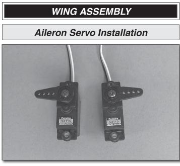
□ 1. Prepare a left and a right servo using your radio system to center the servos. Remove the servo arm retaining screws and the servo arms. Install the standard size servo arms that came with your servos. Rotate the arm on the splined servo shaft and choose the arm that is 90° to the side of the servo case when the servo is centered. Clip off the unused servo arms so that your aileron servos appear as shown. Fit any servo grommets now (if equipped).
