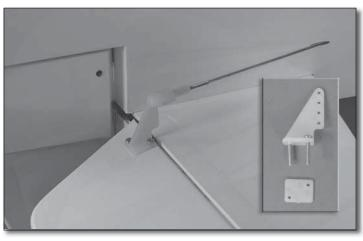
$\Box$  5. Install the control horn using the backing plate and two 2-56 x 1/2" [12.7mm] machine screws. Fit the clevis to the outermost hole in the control horn.
