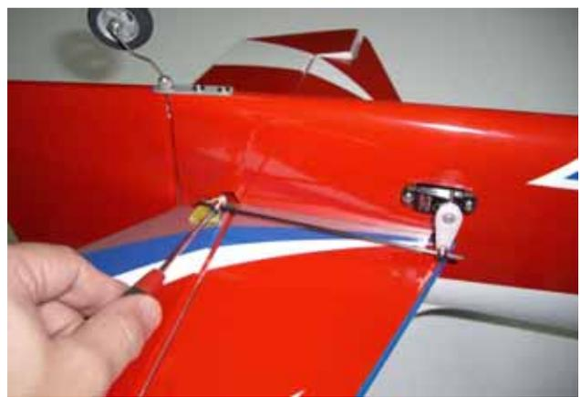
**Section 6 – rudder servo & control horn installation**
