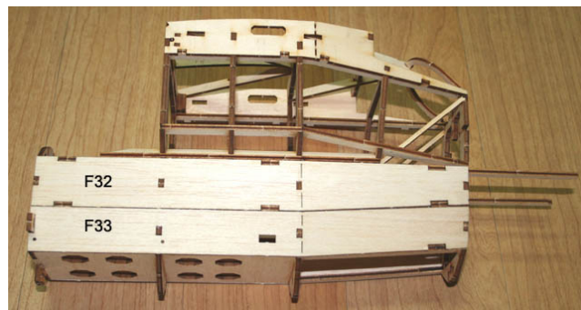
12. Cover the sheets(F32-F33) with thick CA.
