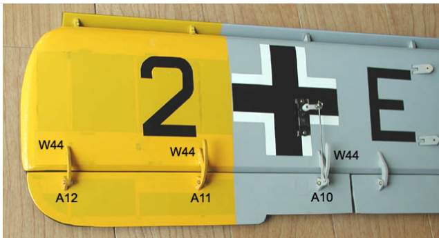
19. This picture shows for 6channel receiver. aileron1, aileron2(mixed), flaps(Y-extension).
