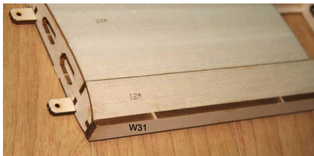
13. Glue leading edge(W31) with thick CA.
