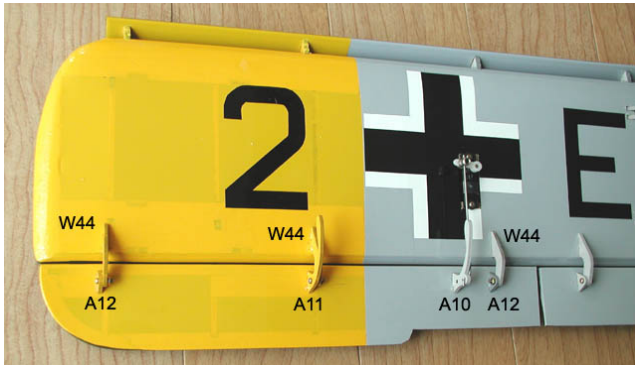
18. Temporarily glue aileron horns (W44) with small amount of CA. After throwing check, and then glue them firmly. Above picture shows for 6channel receiver. aileron(Y-extension), flaps(Y-extension)
