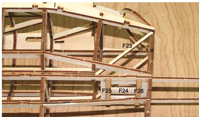
7. Assemble and glue the parts(F23-F26) with thick CA.
