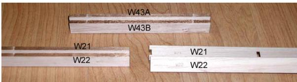
16. Glue the slat parts together (W21-W22, W43A-W43B) with thick CA.
