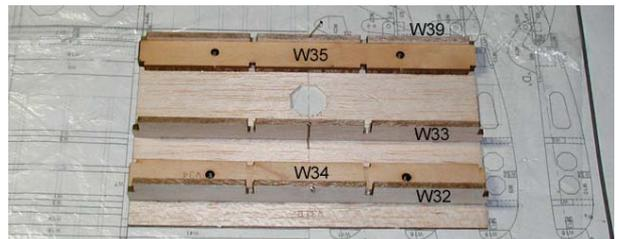
11. Pin the lower sheet(W31A, W31B) and temporary assemble spars, trailing edge(W32, W33, W39) and balsa(below) and plywood(above) wingbolt mounts(W34's, W35's).
