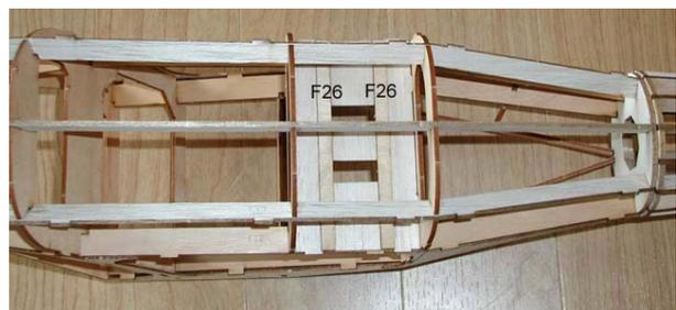
11. Glue plywood servo rails(F26).
