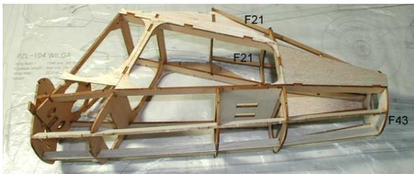
5. Install the part(F21) and bulkhead(F43). Pins and glues are not required in this step.
