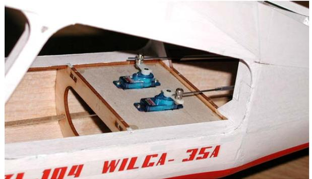
19. Install elevator and rudder servos.
