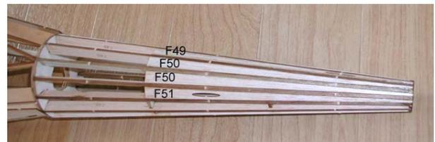
10. Install panels for pushrod exit(F49-F51). **Apply thick CA glue at each joints for reinforcing.** Insert and glue plastic pipes for elevator and rudder pushrods.
