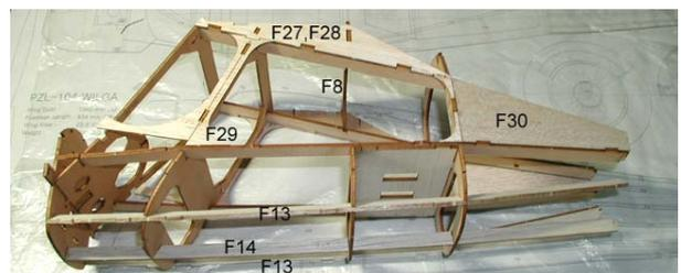
4. Install bulkhead(F8), left side parts(F27, F28, F29, F30) and lower longerons(F13, F14).
