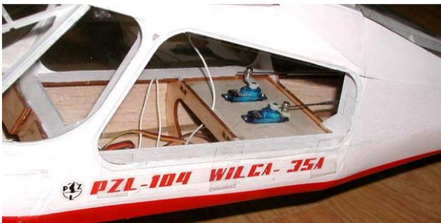
26. Cut clear plastic left side windshield, attach with clear tape. (This window should be a hatch for battery and your maintenance.)
