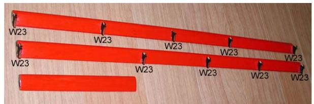
2. Insert and glue plywood slat supports(W23).
