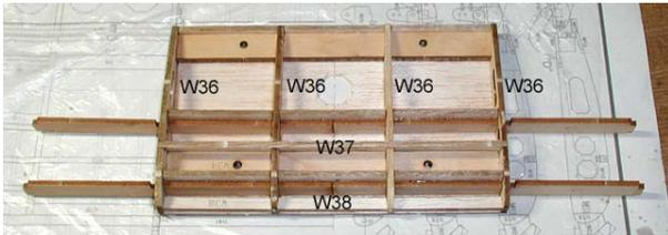
13. Assemble ribs(W36), spar(W37), sub leading edge(W38) and then, glue them.
