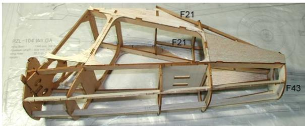
5. Install the part(F21) and bulkhead(F43). Pins and glues are not required in this step.
