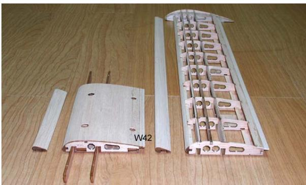
18. Glue center trailing edge(W42) with thick CA. **Apply thick CA glue at each joints for reinforcing.** And then, carefully sand surfaces.
