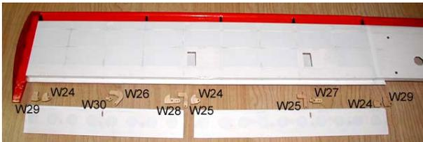
7. Prepare aileron and flap hinges and horns(W24-W30).
