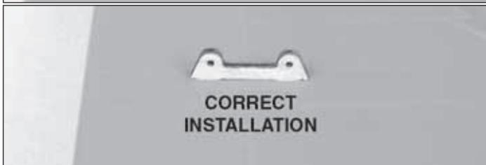
❑ 2. Grab the two strut mounts that you marked "A" and insert them into the pockets on the top wing as shown. They are designed to fit only one way. If you observe a large gap between the wing and strut mount, remove it and try it the other way. **DO NOT** glue them into place at this time.
