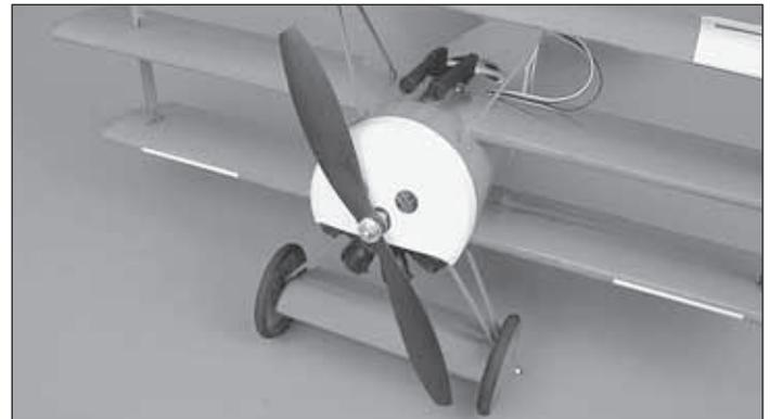
❑ 3. Install a 10" x 4.5" propeller. Install the prop washer and prop nut and tighten the nut securely.
