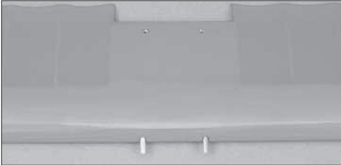
❑ 1. Locate two of the 3mm x 24mm [1/8" x 15/16"] dowel rods and insert them into the bottom wing as shown, so that only about 9mm [11/32"] sticks out. Secure them with medium CA.
