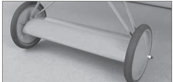
❑ 4. On each end of the axle, place a 3mm [1/8"] washer and 3mm [1/8"] nut with threadlocker, followed by another 3mm [1/8"] washer and the wheel. Secure the wheel in place with a 3mm [1/8"] washer and 3mm [1/8"] nut. Apply a drop of threadlocker to the nut.
