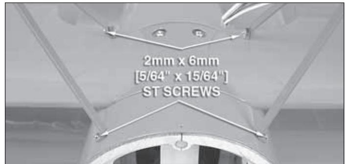
❑ 4. Locate the two cabanes and install them as shown using four 2mm x 6mm [5/64" x 15/64"] self-tapping screws as shown. Remove the screws and apply a couple of drops of thin CA into each hole to harden the threads. Re-install the cabanes.
