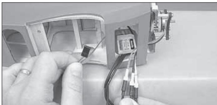
❑ 3. Cut a 20mm [3/4"] long piece of hook and loop material (not included). Glue the 20mm [3/4"] soft piece (loop side) to the back of the ESC. Glue the rough piece (hook side) to the side of the fuse, next to the battery tray. Insert the ESC into the battery door and through the cut-out just to the rear of the firewall and secure it in place by joining the hook and loop material. Route the servo lead into the wing opening area and the three motor leads out the front of the firewall.
