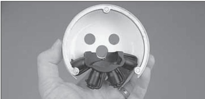
❑ 2. Use Medium CA to glue the dummy engine in place on the cowl as shown.
