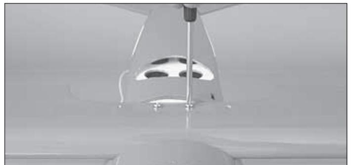
❑ 2. Place the middle wing on the wing saddle as shown and secure it with two 3mm x 24mm [1/8" x 15/16"] machine screws and 3mm [1/8"] washers. The flat side of the wing is the bottom.
