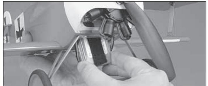
❑ 1. Cut a 20mm [3/4"] long piece of hook and loop material (not included). Glue the rough piece (hook side) to the battery tray. Glue the 20mm [3/4"] soft piece (loop side) to the back of the battery pack. Insert the battery into the battery compartment and secure it in place by joining the hook and loop material.
