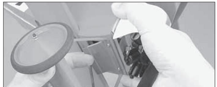
❑ 2. Put the battery cover in place. Note that the lip slides into the fuse and the aft end is held on with two magnets.
