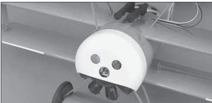
❑ 1. The cowl is held on with three small but powerful magnets. Put the cowl in place so that the motor shaft is centered in the opening as shown.
