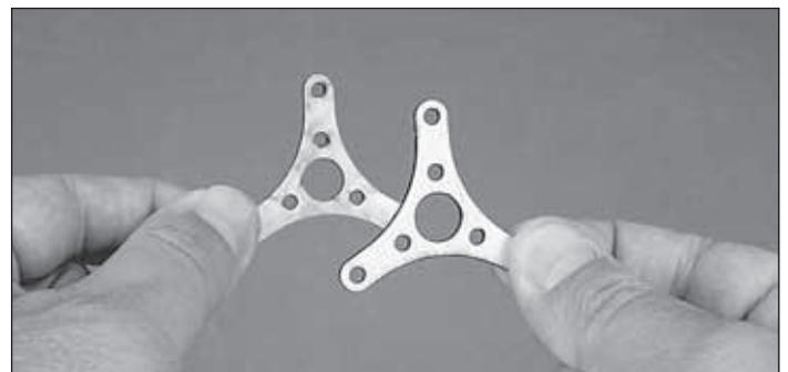
❑ 1. Use epoxy to join the two piece motor mount. Make sure all openings align.
