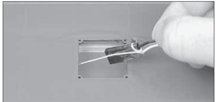
**TIP:** After tying the string to the right aileron servo plug, use tape to keep the string and plug headed in the same direction. This accomplishes two things; it keeps the plug from doubling back over itself and keeps the string securely fastened to the plug.
