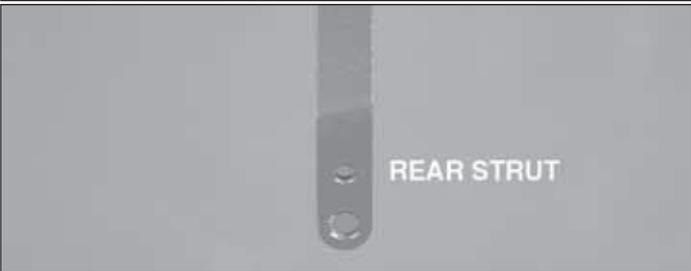
❑ 1. Carefully thread the axle through the sub-wing and attach the rear landing gear strut followed by the front landing gear strut as shown. The rear strut is identified by a second hole near the axle hole.
