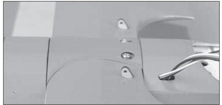
❑ 3. Grab the two strut mounts that you marked "B" and insert them into the pockets on top of the middle wing as shown. **DO NOT** glue them into place at this time.
