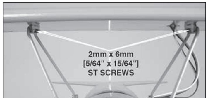
❑ 5. Put the top wing in place atop the cabanes and secure it with four 2mm x 6mm [5/64" x 15/64"] self-tapping screws. Remove the screws and apply a couple of drops of thin CA into each hole to harden the threads. Re-install the top wing.
