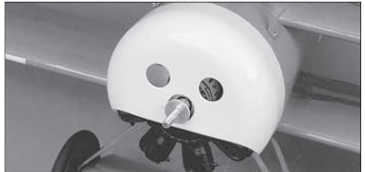
❑ 2. Slide the prop shaft and collet onto the motor shaft. The collet has a tapered hole through it.
