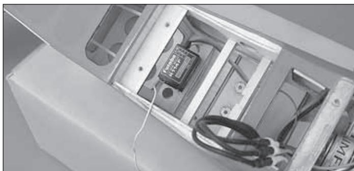
❑ 5. Cut another 20mm [3/4"] long piece of hook and loop material (not included) and glue the 20mm [3/4"] soft piece (loop side) to the back of the receiver. Glue the rough piece (hook side) to the top of the inside of the fuse on the ledge by the cockpit opening. Insert the receiver and secure it in place by joining the hook and loop material.
