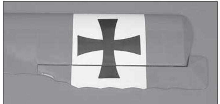
❑ 2. Remove any pins you may have inserted into the hinges. Install the aileron so there is a very small gap between the LE of the aileron and the wing. The gap should be small – just enough to see light through or to slip a piece of paper through.
