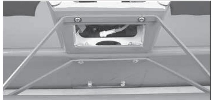
❑ 3. Attach the landing gear to the bottom of the fuse with four 2mm x 7mm [5/64" x 9/32"] self-tapping washer head screws. Remove the screws and harden the holes with thin CA. Then, reinstall the screws.
