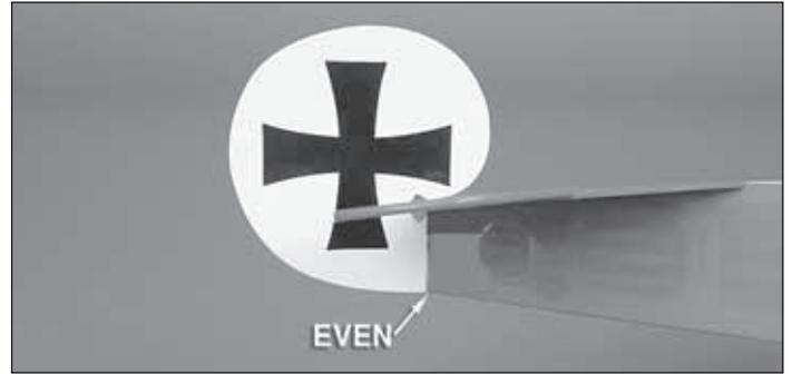
❑ 10. Install the 10mm x 21mm [3/8" x 13/16"] CA hinge in the rudder and test fit it into the rear of the fuse. Adjust the rudder so that the bottom is even with the bottom of the fuse. Use a small modeling square to make sure that it is perpendicular to the stab. Apply 3 drops of thin CA on each side of the hinge.
