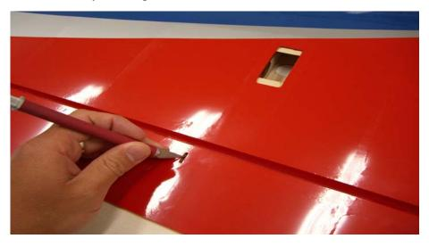
Place the fibreglass horn into aileron, check for correct alignment and glue it with some drops of medium CA.
