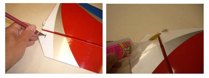
Install the elevator carbon tube, and using the provided two screws and washer install the stabilizer.
