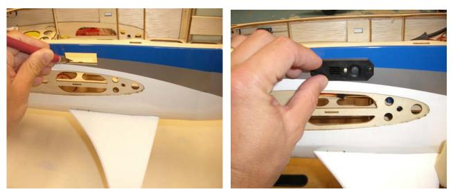
Locate and install the switch with a Phillips screwdriver as follow.
