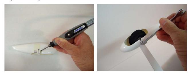
Hold the wheel pant parallel to the fuselage and drill the location for the wheel pant screw using a 1,5mm drill bit. Attach the wheel pant to the landing gear using a 2mm short self-tapping screw.
