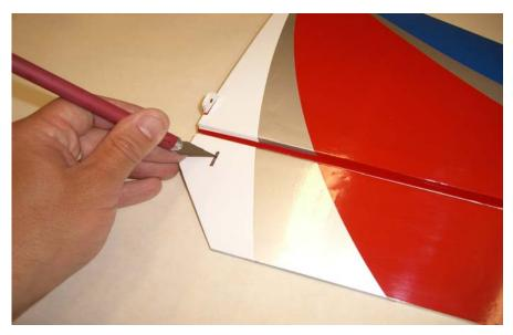
Place the fibreglass horn into elevator, check for correct alignment and glue it with some drops of medium CA.
