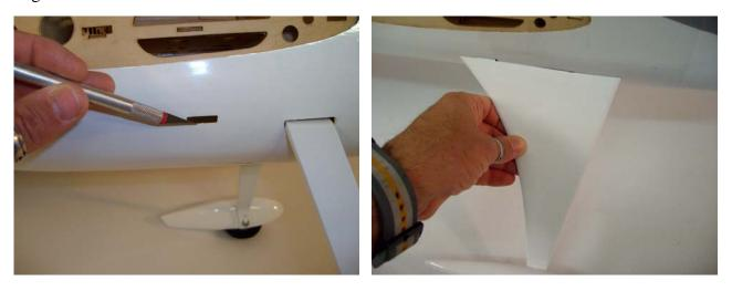
Once satisfied with the fit, glue the fillet on the landing gear using medium CA. Use the glue carefully avoid over runs on other areas.
