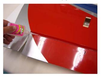
Work the aileron up and down some times to work the hinges and check for proper movement.
