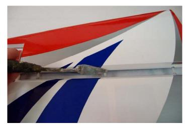
Work the elevator up and down some times to work the hinges and check for proper movement.
