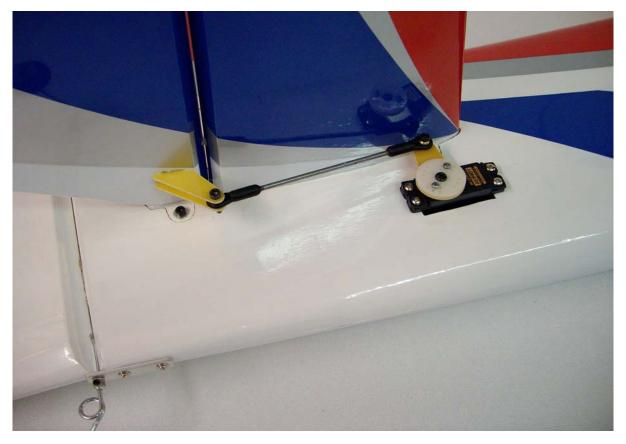
When you like to install again the F3A elevators, remove the 3D elevator with control horns and servo arms and the carbon tube, as follow.
