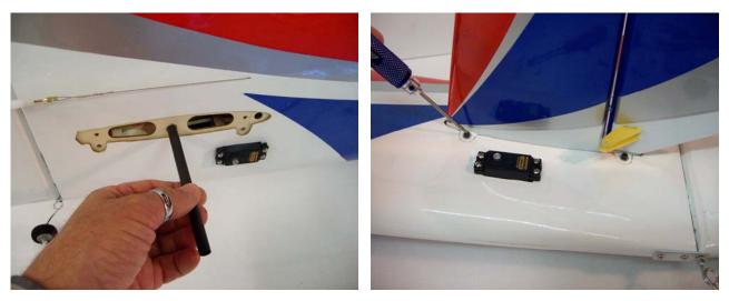
□ step 10 Install the hardware and make the final adjustment as per picture.
