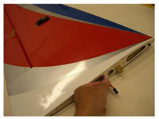
□□ **step 6** Install the control horn as per picture.
