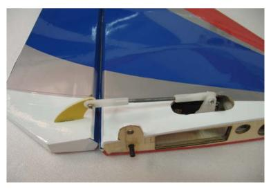
Install the elevator on the fuselage, with the two screws and washer included in the hardware pack.
