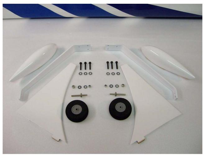
Using screws and washers, install the landing gear as follow.
