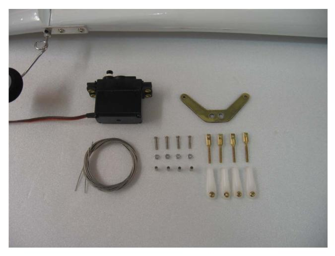
Drill the location for the four self-tapping screw using a 1.5mm drill bit and install the servo as per the picture.
