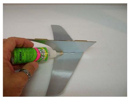
With the hobby knife open the two slots on top fuselage and carefully glue the fin with medium CA.
