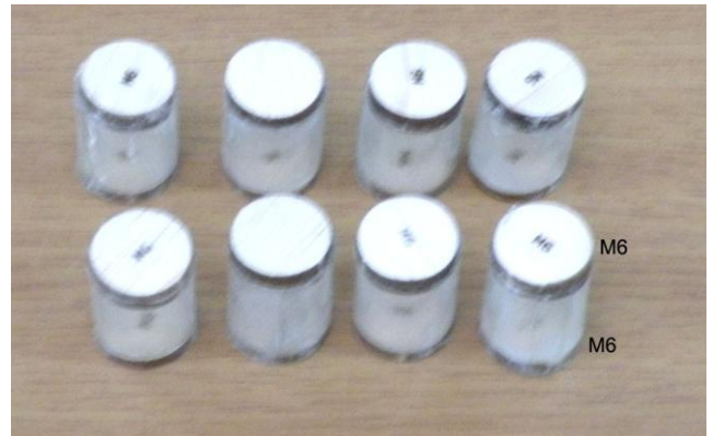
3. Roll up PVC film to the parts(M6) for dummy engine cylinders. (Refer to dummy engine cylinder template on the drawing.)
