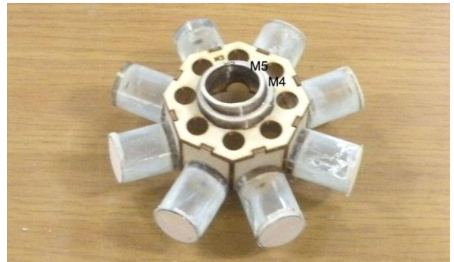
4. Glue dummy engine cylinders to crank case.
