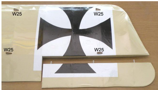
8. Glue the parts(W25), make aileron hinge slots and then install hinges.
