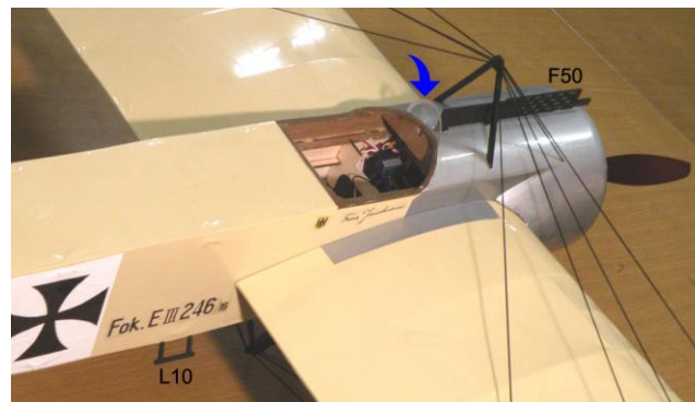
19. Glue windshield, step(L10) and machine gun(F50). (Refer to windshield template on the drawing.)
