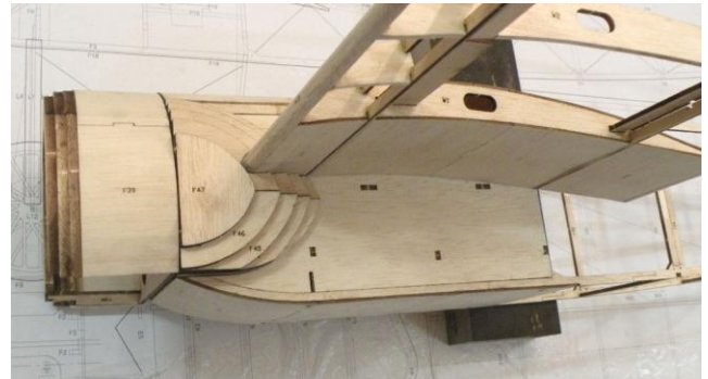
18. Assemble and glue parts(F40-F42) as shown above.
